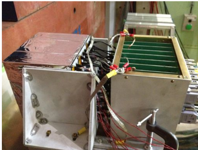
Figure 12.12: The prototype electron calorimeter system consisting of 7 \times 7 GSO crystals.
