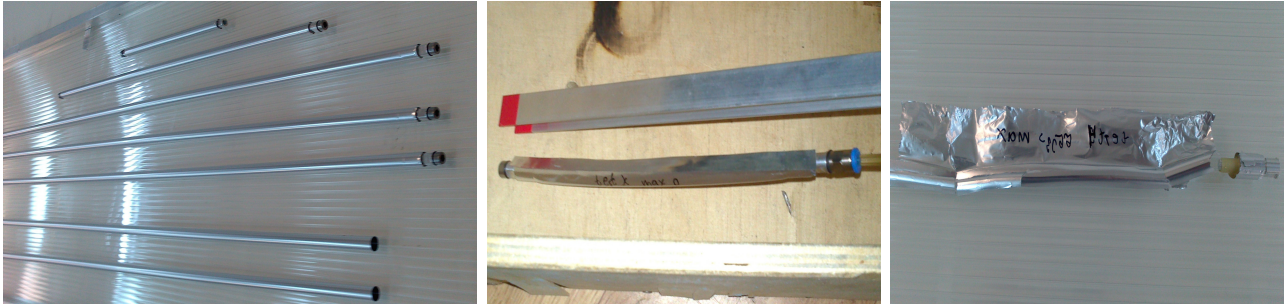
Figure 11.6: The latest achievement of thinner straw tube R&D; (Left) Sample tubes of 20 \mu\text{m} thick wall with 70 nm aluminium deposition, (Centre) Over-pressurise test with 6 bar, (Right) Over-pressurise test with 7.5 bar
