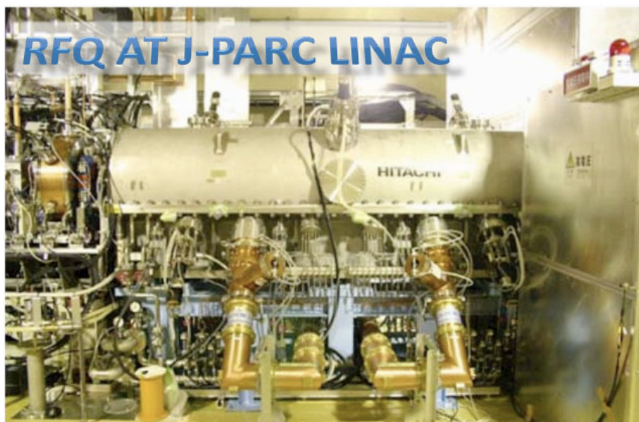
Figure 1.9: Existing RFQ at J-PARC Linac. We plan to use the second spare of the same design.
