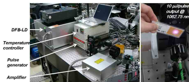
Figure 4.23: DFB-LD + Fiber Amplifier system for 1062.75 nm
